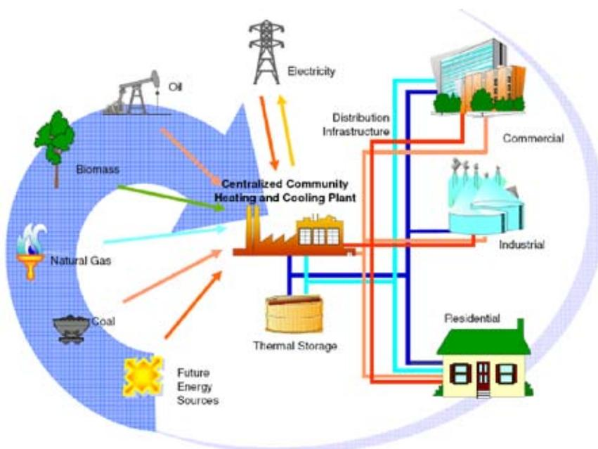
As can be seen from above the district energy system is very flexible in terms of fuel / energy source, it is able to serve numerous customers at the same time and last but not least it has the potential of storing the energy (thermal storage).
